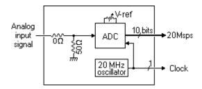
The input on the left is analog, while the outputs on the right are digital.
