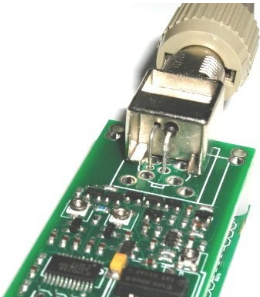
Illustration 1: BNC right-angle mounting position 1
