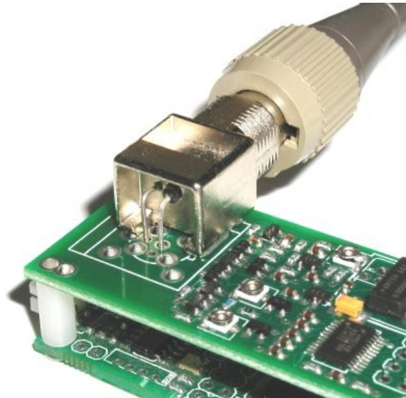
Illustration 2: BNC right-angle mounting position 2
